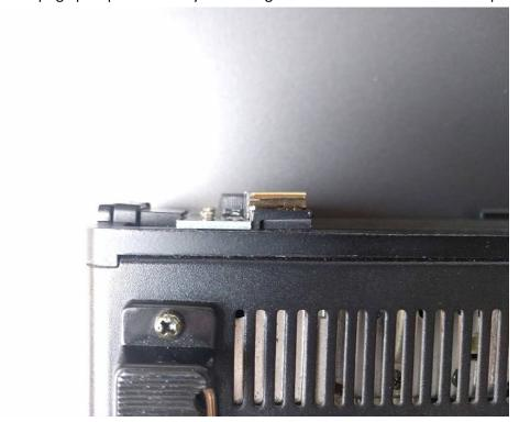
5. Insert a head unit adapter until it is fixed with original locker:
