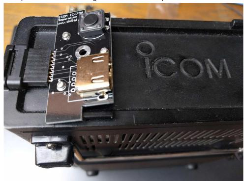
2. Push the base unit adapter and fix it with a thumb screw:
